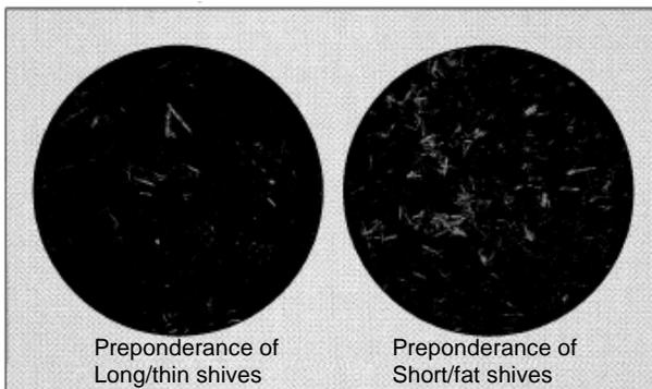
**Figure 2: Good and Poor shive characteristics in groundwood**
