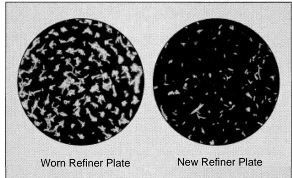
**Figure 3: Good and Poor shive characteristics in TMP.**
